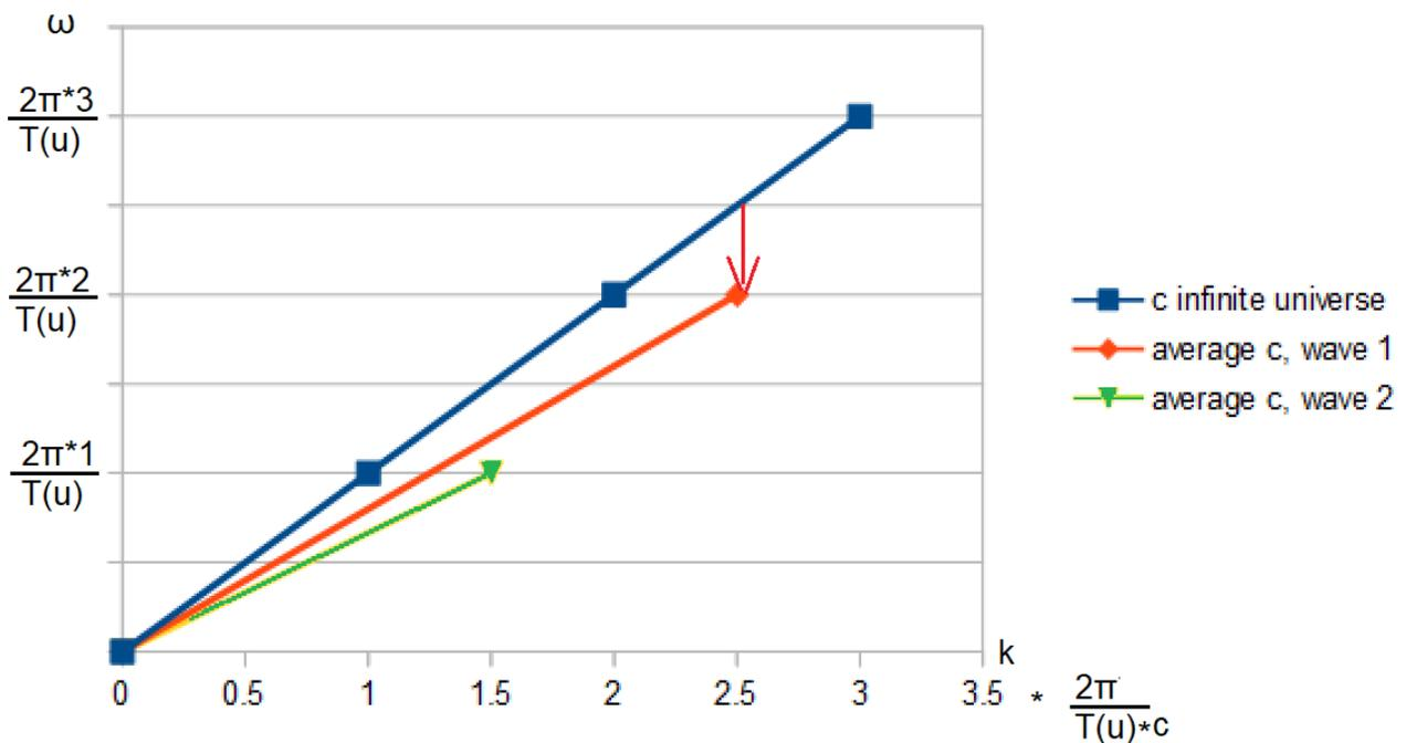
For the wavelength marked red with  $\lambda = 2.5 \cdot c \cdot T_u$ , the frequency  $2.5 / T_u$  would actually be provided for a continuous frequency range. However, since only discrete values are allowed for the frequencies ( $n / T_u$ ,  $n$  natural number), it must be rounded down to  $2 \cdot c \cdot T_u$ , because at  $f = 3 \cdot c \cdot T_u$  the wave would have faster than light speed.
