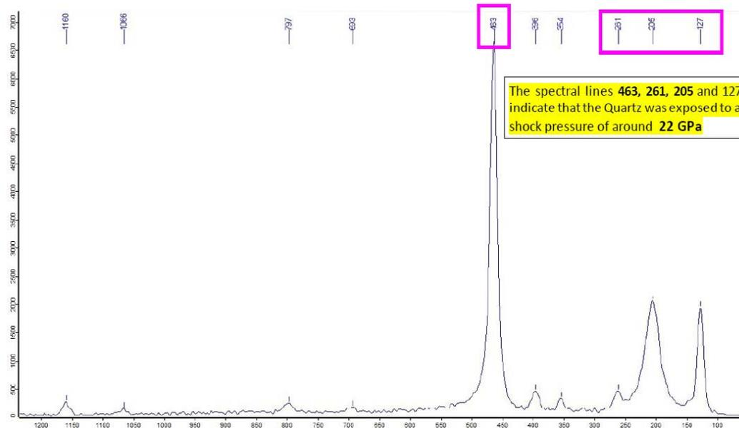
Indication for a shock event are the shifts of the marked Quartz spectral lines towards **261 and 205**
