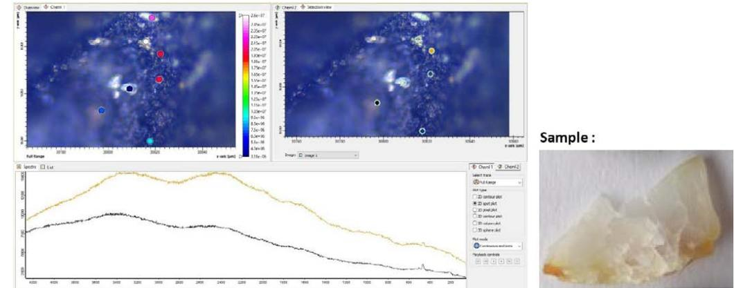
Indication for a shock event are the shifts of the marked Quartz spectral lines towards **463, 260 and 205**
