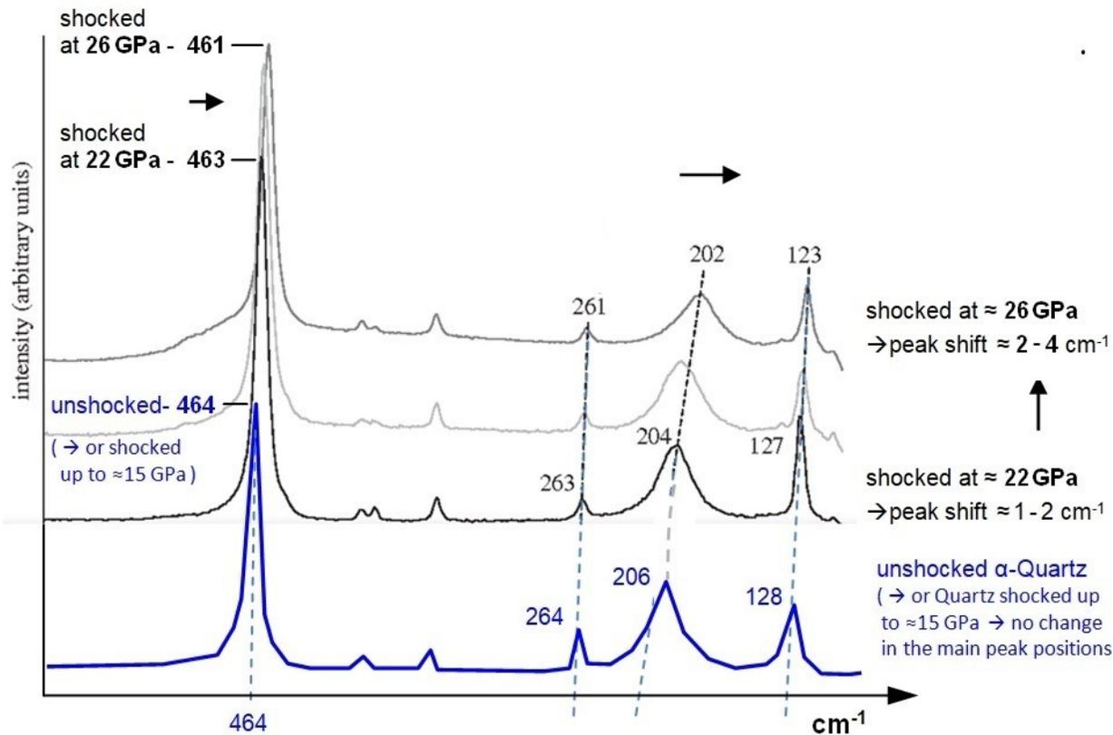
**Quartz shocked with 22 GPa and 26 GPa** → shows shifts of the main RAMAN-peaks of 1 - 4 cm<sup>-1</sup> towards lower frequencies , compared with unshocked Quartz
