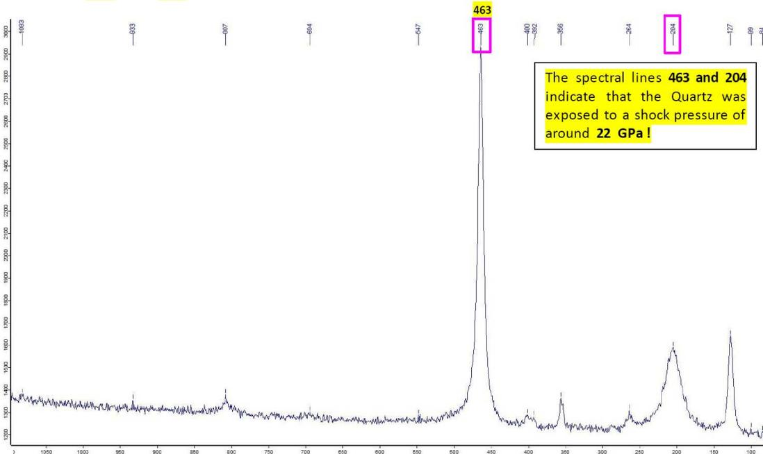
Indication for a shock event are the shifts of the marked Quartz spectral lines towards **263** and **205**
