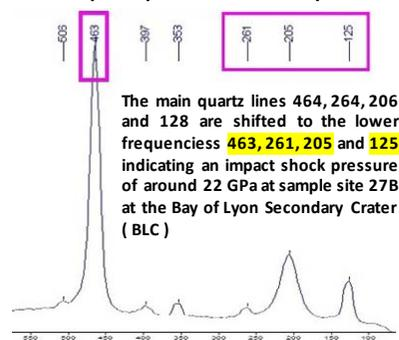
The main quartz lines 464, 264, 206 and 128 are shifted to the lower frequencies 463, 261, 205 and 125 indicating an impact shock pressure of around 22 GPa at sample site 27B at the Bay of Lyon Secondary Crater (BLC)
