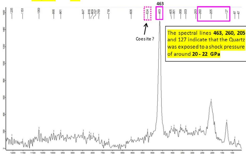
Indication for a shock event is the shift of the marked main Quartz spectral line towards **463**
