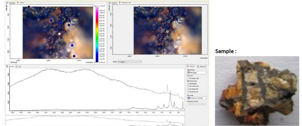
Indication for a shock event are the shifts of the marked Quartz spectral lines towards **463**, **260** and **204**
