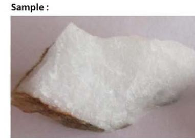
The spectral lines **463, 260 and 205** indicate that the Quartz was exposed to a **shock pressure of ≈ 22 GPa**
