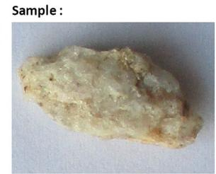
The shift of the main spectral line of Quartz towards **463** in the sample indicates a shock pressure of around **22 GPa**
