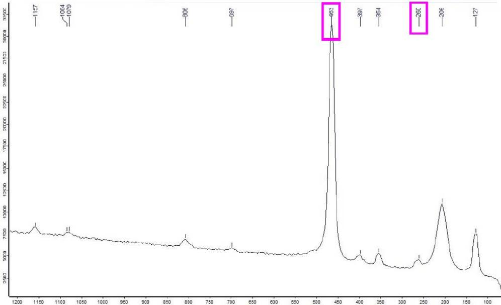
Indication for a shock event is the shift of the marked Quartz spectral line towards **205**
