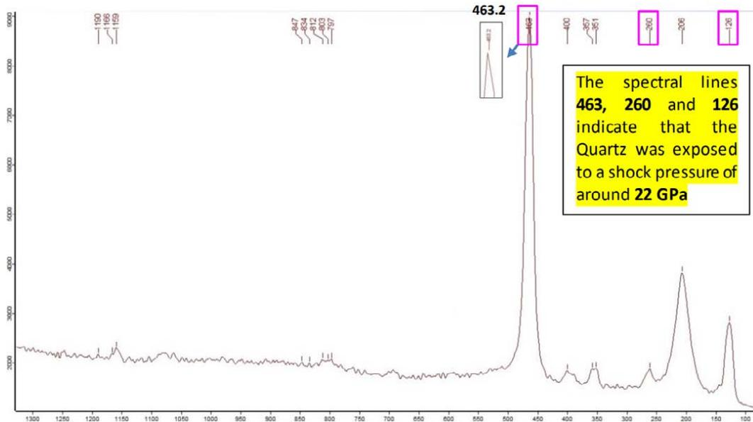
Indication for a shock event are the shifts of the marked Quartz spectral lines towards **463, 261, 203** and **126**
