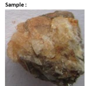
Indication for a shock event are the shifts of the marked Quartz spectral lines towards **463, 261, 198 and 125**
