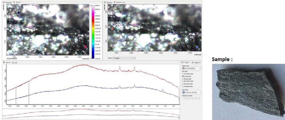
Indication for a shock event is the shift of the marked Quartz spectral line to **463**
