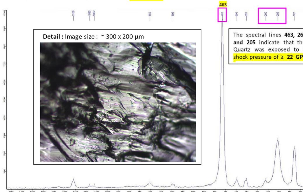
The spectral lines **463, 261, 205 and 125** indicate that the Quartz was exposed to a **shock pressure of ≈ 22 GPa !**
