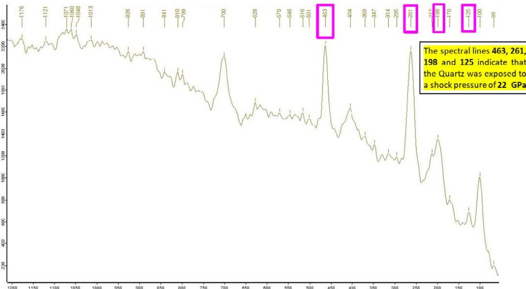
Indication for a shock event are the shifts of the marked Quartz spectral lines towards **463, 262 and 205**
