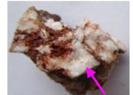
Indication for a shock event are the shifts of the marked Quartz spectral lines towards **463, 260** and **126**
