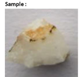
Indication for a shock event are the shifts of the marked Quartz spectral lines towards **463, 261 and 205**
