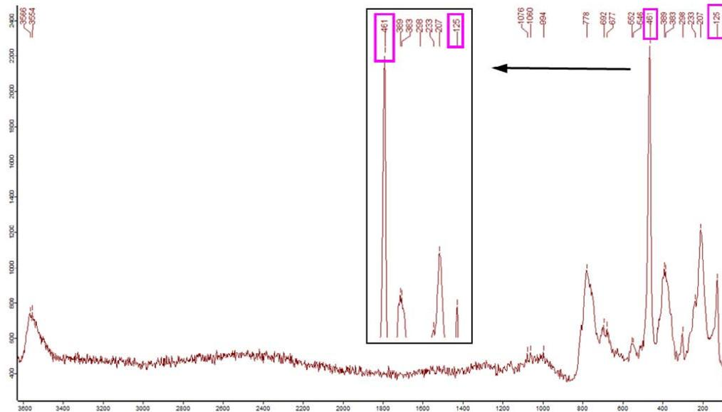
The shift of the main spectral line of the Quartz towards **463, 261, 205 and 125** in the sample indicates a shock pressure of around **22 GPa**
