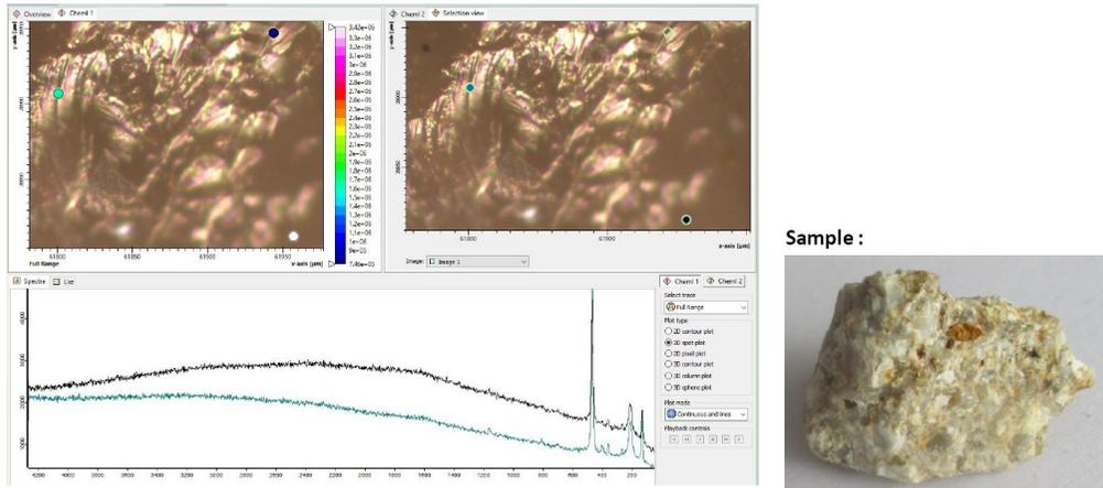
Indication for a shock event are the shifts of the marked Quartz spectral lines towards **261** and 201 (209)
