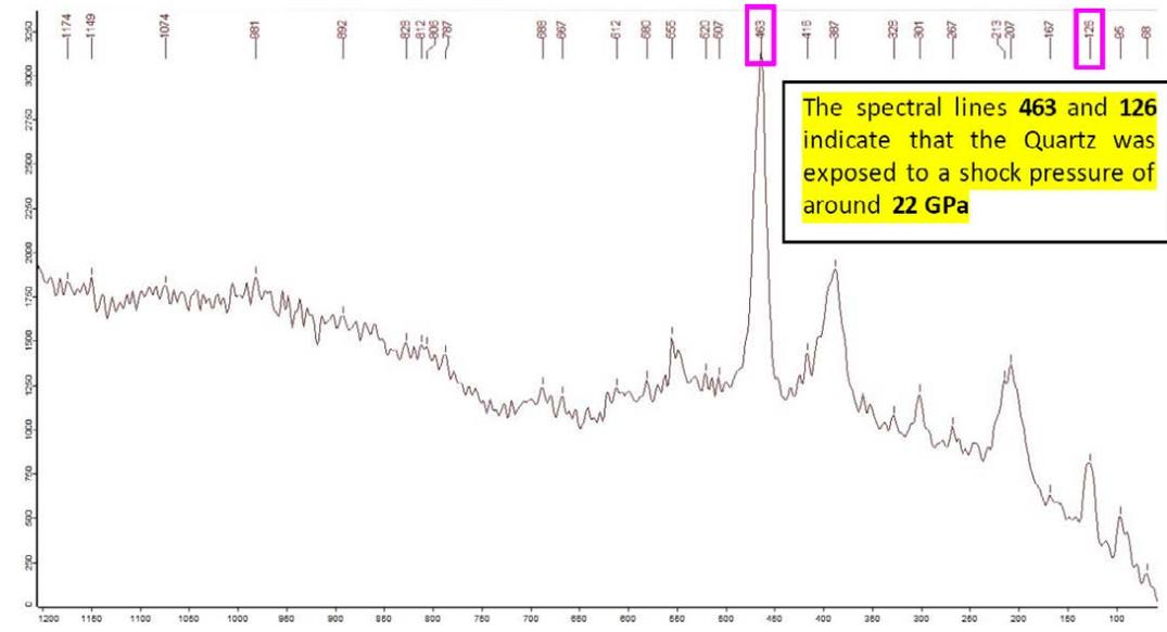
The spectral lines **463** and **126** indicate that the Quartz was exposed to a shock pressure of around **22 GPa**
