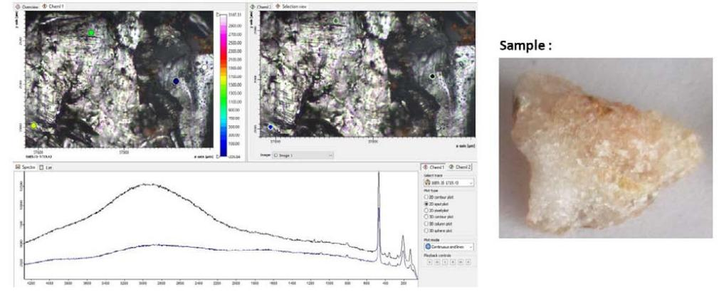
The spectral lines **463, 262/268 and 125** indicate that the Quartz was exposed to a **shock pressure of ≈ 22 GPa**
