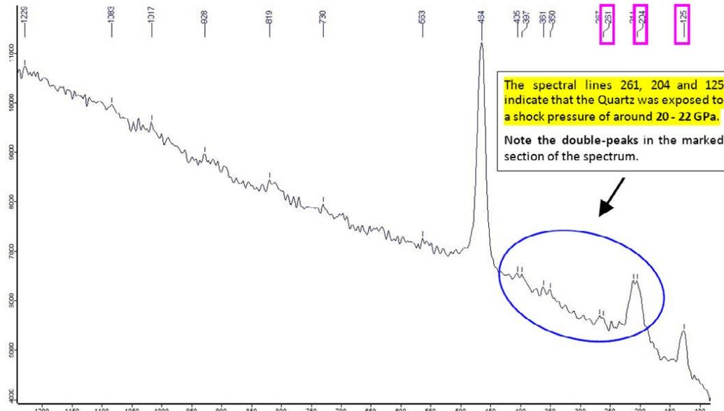
Indication for a shock event are the shifts of the marked Quartz spectral lines towards **260** and **205**
