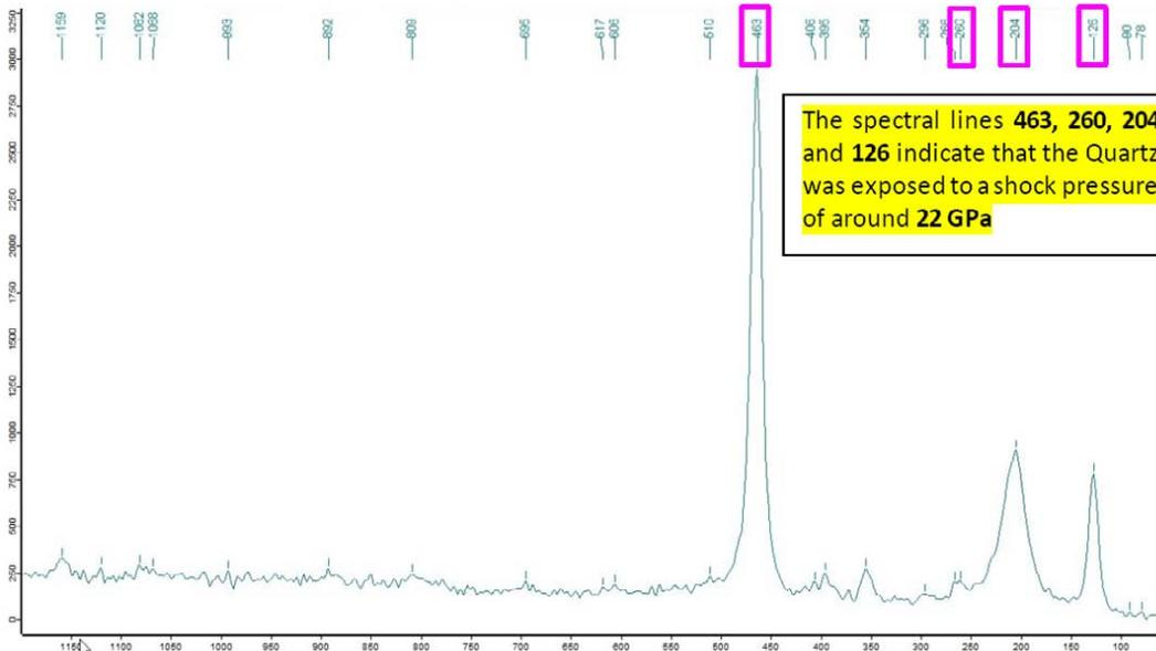
The spectral lines **463**, **260**, **204** and **126** indicate that the Quartz was exposed to a shock pressure of around **22 GPa**
