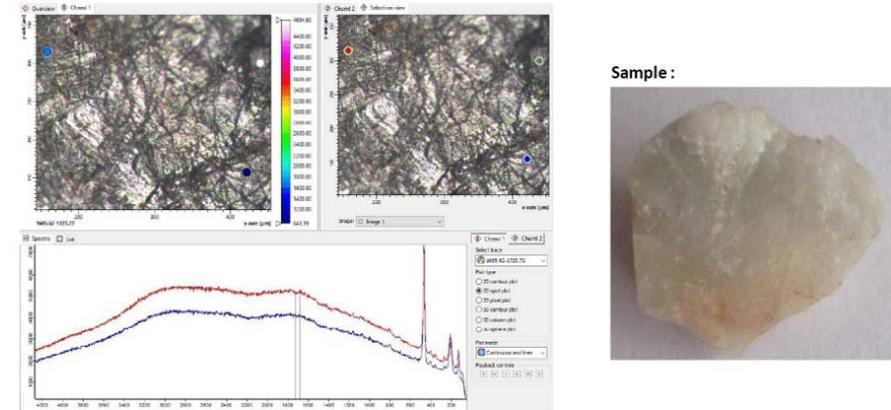
The spectral lines **463, 261, 204 and 126** indicate that the Quartz was exposed to a **shock pressure of ≈ 22 GPa**
