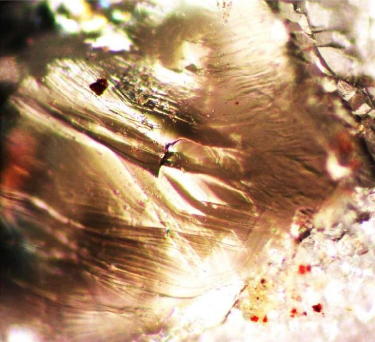
Indication for a shock event are the shifts of the marked Quartz spectral lines towards **263** and **205**
