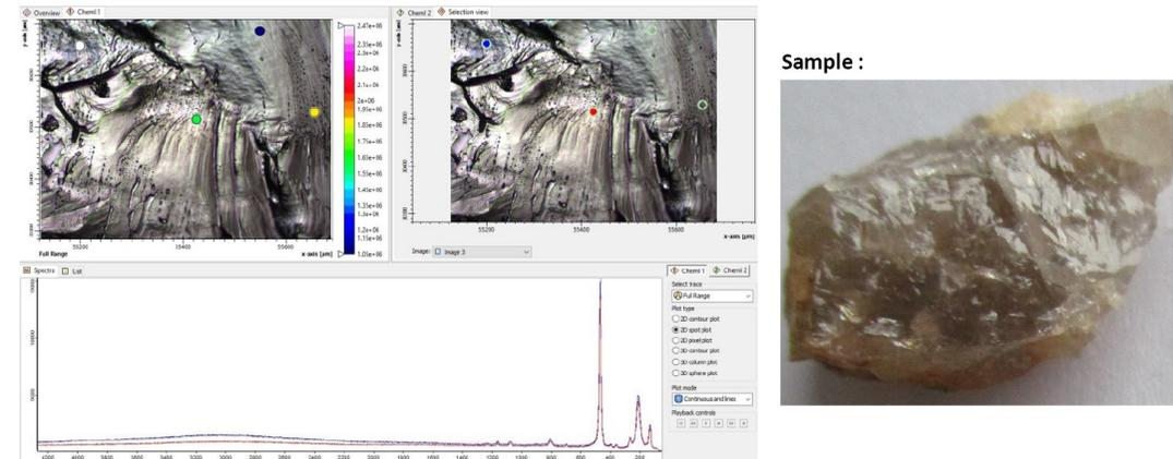
The spectral lines **463, 258/264, 205 and 126** indicate that the Quartz was exposed to a shock pressure of around **22 GPa!**
