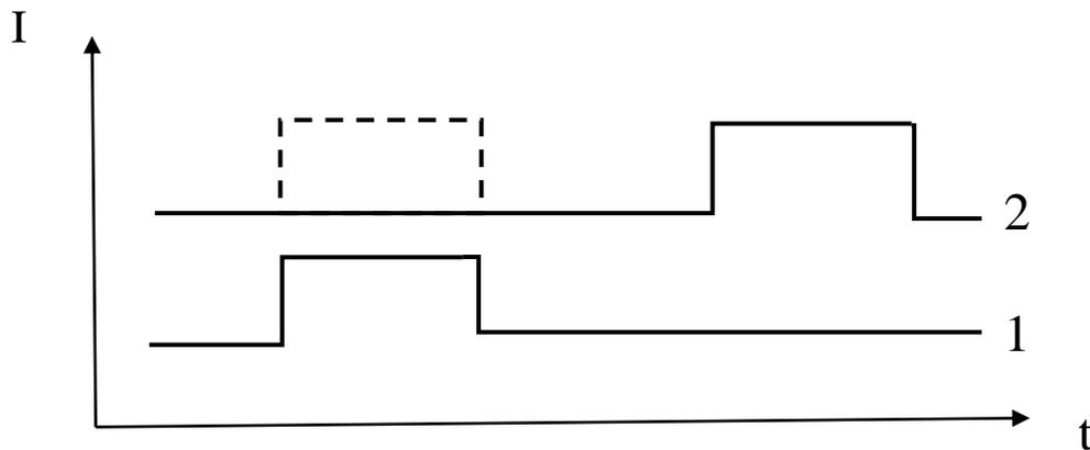
**Figure 2.** The expected results of the experiment. 1 - oscillogram of the voltage applied to the optical shutter. 2 - radiation intensity recorded by the detector.
