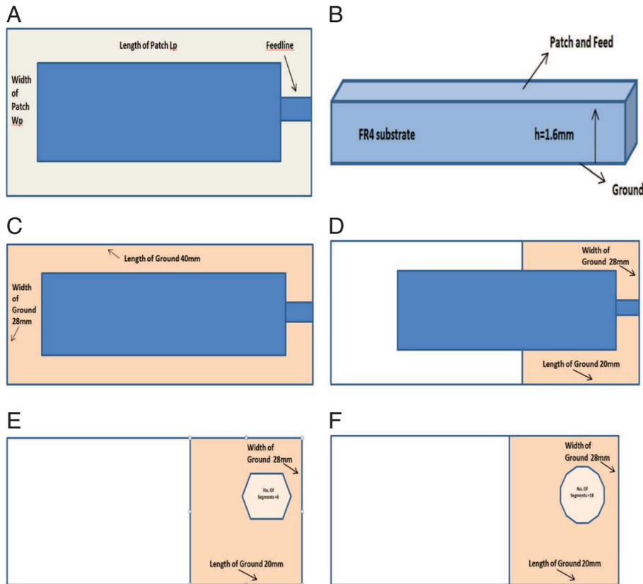
Figure 1: Geometry of the antenna. (A) Top view of the rectangular-patch antenna (RPA), (B) side view of RPA, (C) RPA with full ground plane, (D) PG-RPA, (E) PSG-RPA1 with a polygon cut with six segments, and (F) PSG-RPA2 with a polygon cut with 18 segments.
