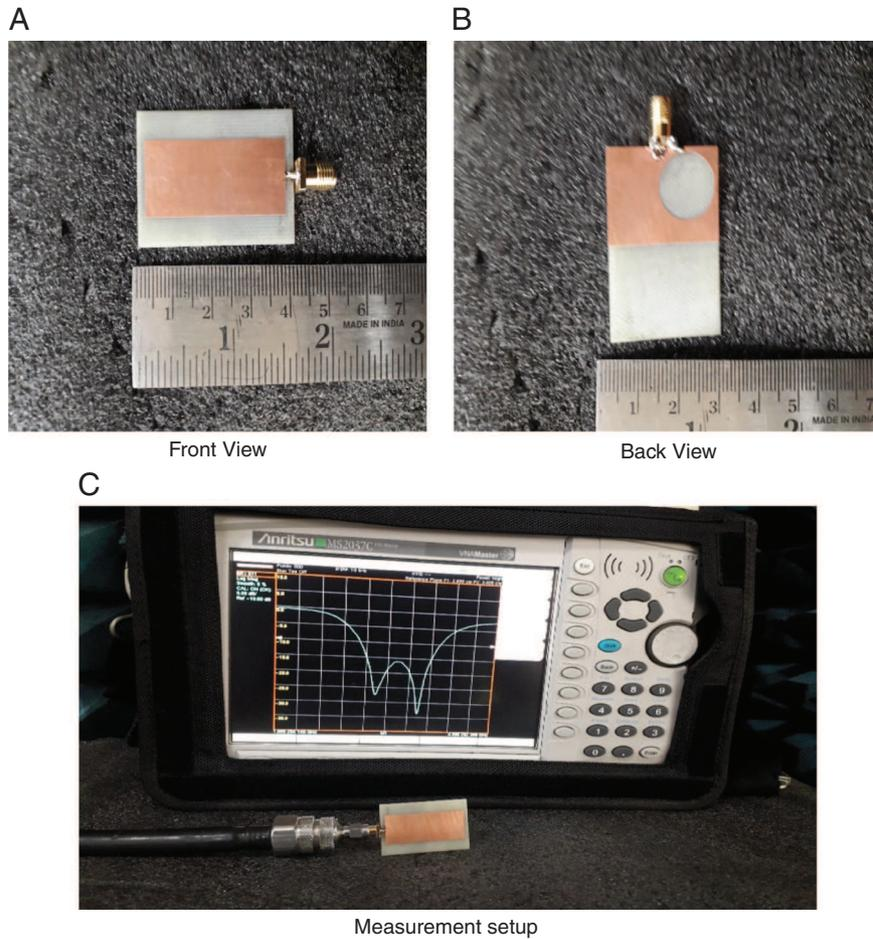
Figure 7: Antenna prototype of PSG-RPA2 (A) front view, (B) back view, and (c) measurement setup.
