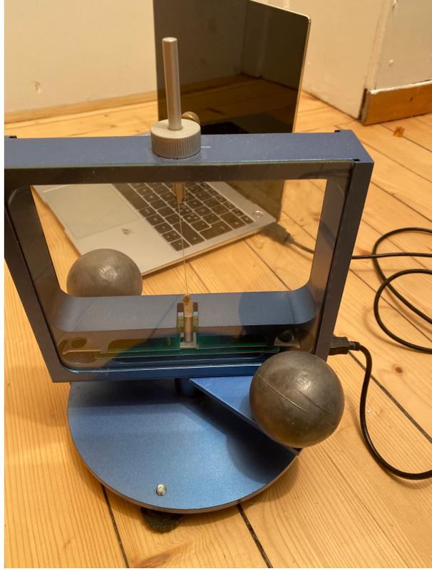
**Figure 1:** Low-budget modern Cavendish apparatus combining old mechanics with modern electronics that feed directly to your computer through a USB cable. It is remarkable that, in using such an instrument, we can measure the Planck mass with only about 5% error.
