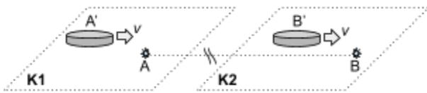
Fig 2. Setup1 to test RoS under first axiom. Moving frame's synchronized detectors at A' and B' pass over the vertical flash sources, A and B to record the time of the flashes in the moving frame.
