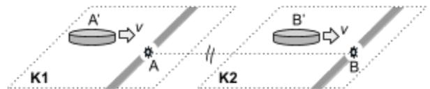
Fig 3. Setup2 to test RoS under first axiom. Moving detectors A' and B' are enabled by spatially limited gray metal strips engraved about A and B for a short duration.
