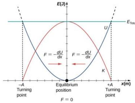
**Figure 4:** Kinetic (K) and potential energy (U) of an oscillator<sup>46</sup>
