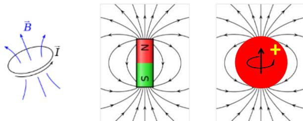
Figure 5a (left). Magnetic field (blue lines) of a current carrying loop (black). Copied from wiki “magnetic field (2016 old version)”. Author: Sbyrnes321 (Steve Byrnes). Copyright: Public Domain.
