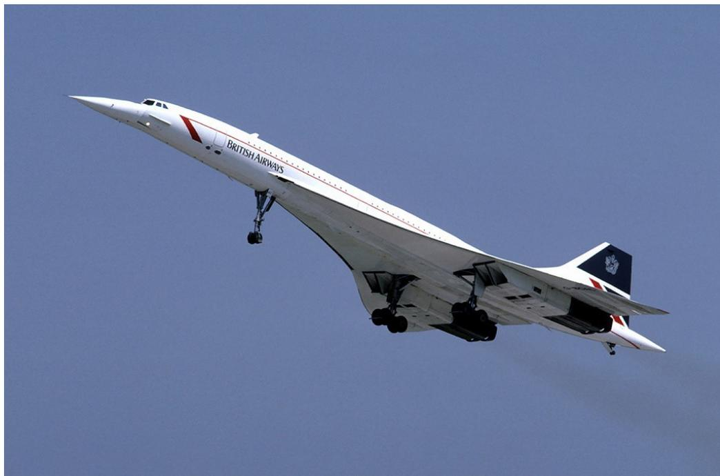
British Airways Concorde G-BOAC. Length 61.66 m, wingspan 25.57 m, wing area 358.6 m<sup>2</sup>, normal take-off weight 187.7 tons, 4×turbojet engines. Aerodynamic quality at  $M=0.94$   $K=11.47$ , at  $M=2.04$   $K=7.14$ .
