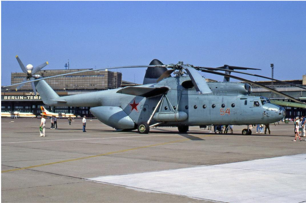
**Mi-6 Helicopter.** 924 helicopters were produced. Load 20 tons, screw diameter of 35 m, the GTE Engines 2 xD-25B. The power of one engine is 250 kW.
