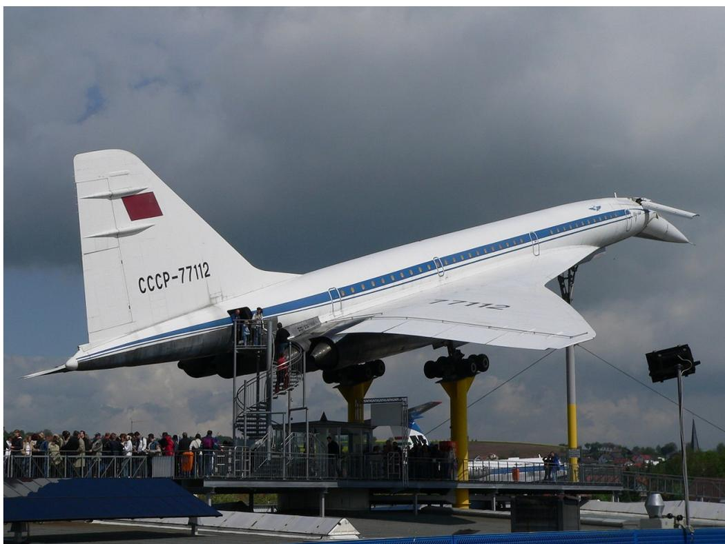
Tu-144 in the Museum in Sinsheim, Germany (No. 77112). Length 65.7 m, wingspan 28 m, wing area 503 m<sup>2</sup>, normal take-off weight 180 tons, engine thrust 4×NK 144A at take-off 4×20 tons.
