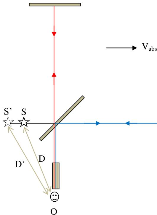
As we can see from the above diagram, absolute motion of the Michelson-Morley interferometer causes only an apparent change in the point of light emission relative to the observer, from S to
