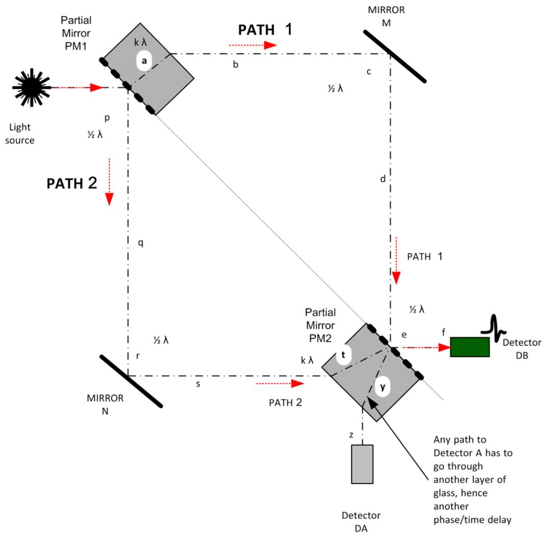
Figure 3: Mach–Zehnder interferometer in default mode. The photon appears at DB.
