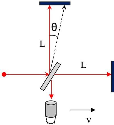
Fig. B1. The Michelson interferometer moves along with the Earth in its motion around the Sun.
