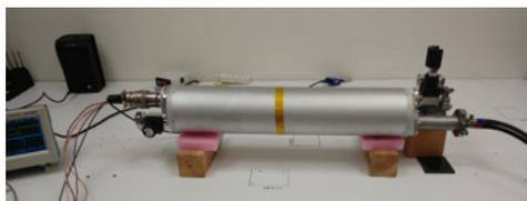
Figure 2: A simple gas detector prototype used in the stability test. Additional fast ionizing-particle “trigger” detectors used to confirm well-timed signals from the gas detector are located below the desk and are not visible in this photo.
