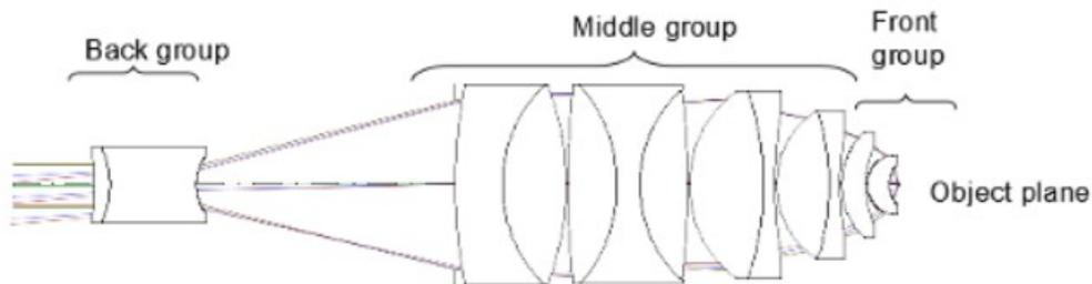
Fig. 3 High NA objectives lens
