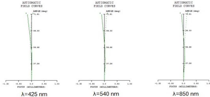
Fig. 5 Flat field objective astigmatism aberration
