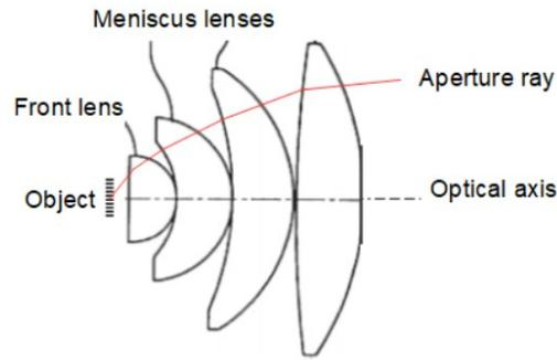
Fig. 2 High NA objective front lens group
