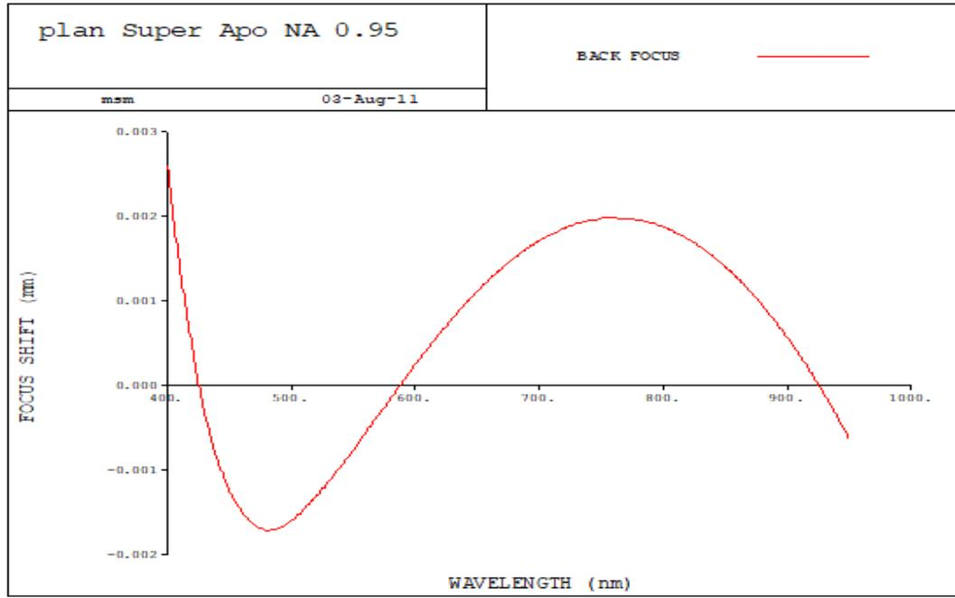
Fig.4 Chromatic aberration curve
