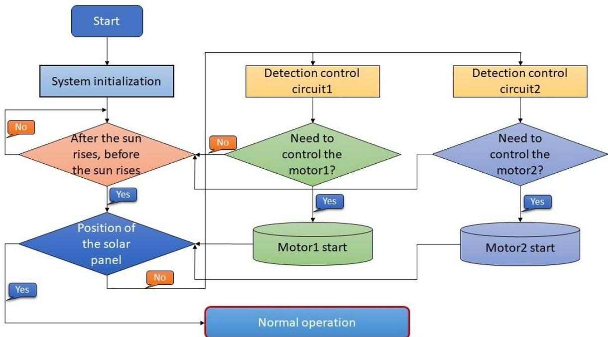
Fig.3. The main flow chart of the sun tracking system
