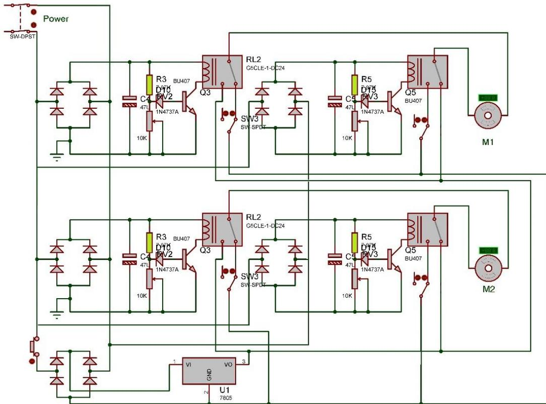
Fig.1. The sensor control circuit for making the solar tracking system
