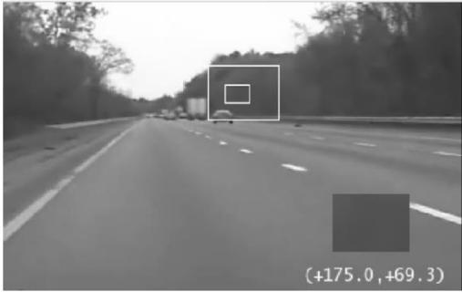
Fig. 13: Vehicle Detection on the road
