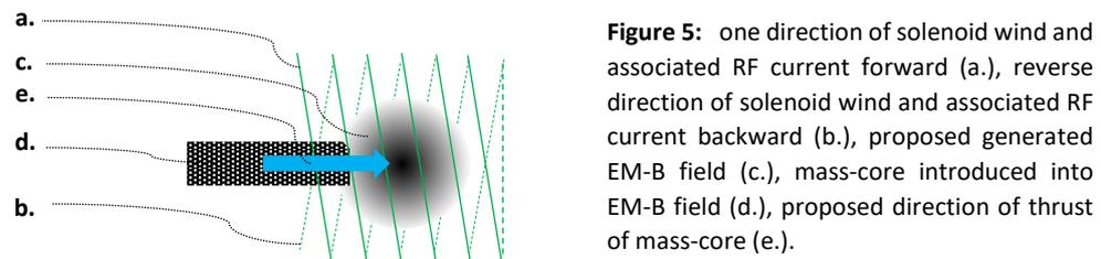
**Figure 5:** one direction of solenoid wind and associated RF current forward (a.), reverse direction of solenoid wind and associated RF current backward (b.), proposed generated EM-B field (c.), mass-core introduced into EM-B field (d.), proposed direction of thrust of mass-core (e.).
