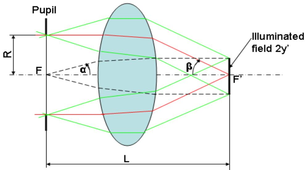
Figure 2. Optical schematic of Transform lens
