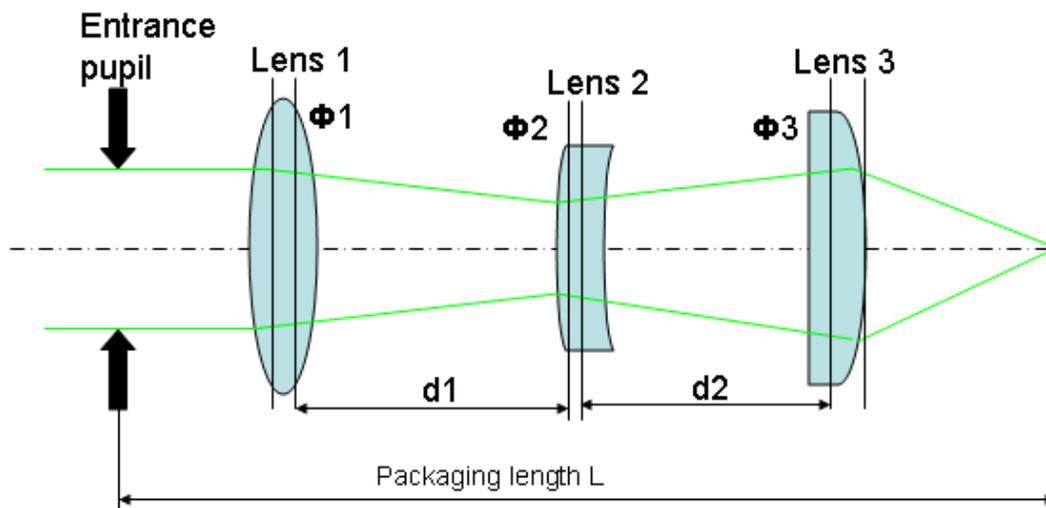
Figure 3. Optical schematic of 3 lens condenser
