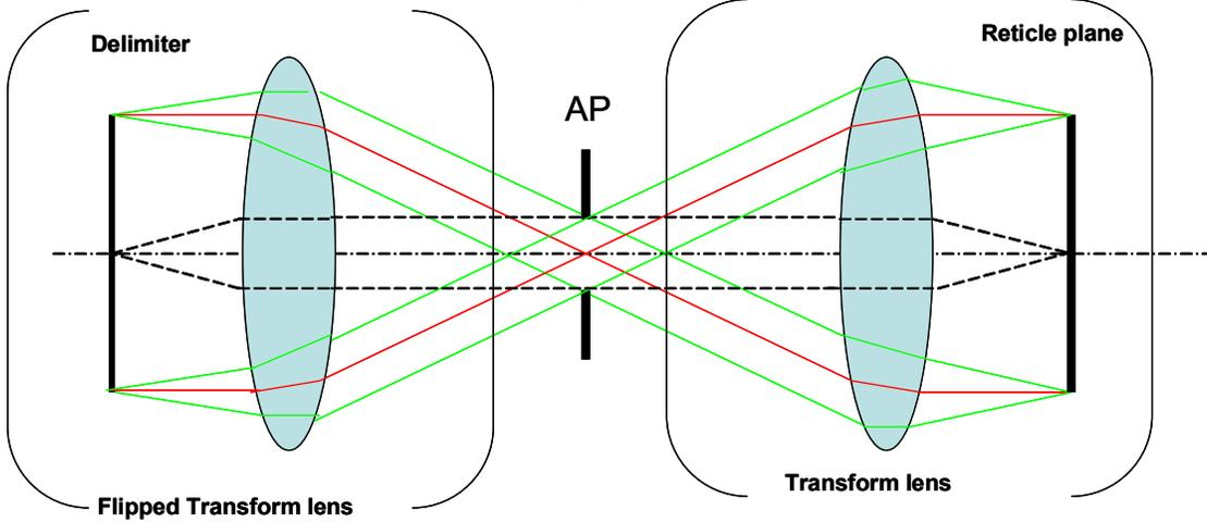
Figure 4. Optical schematic of Relay lens
