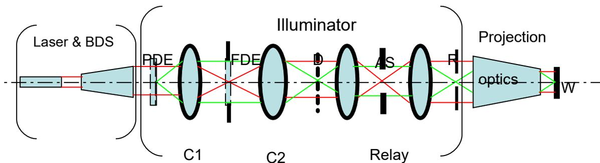
Figure 1 Optical schematic of the typical Litho tool
