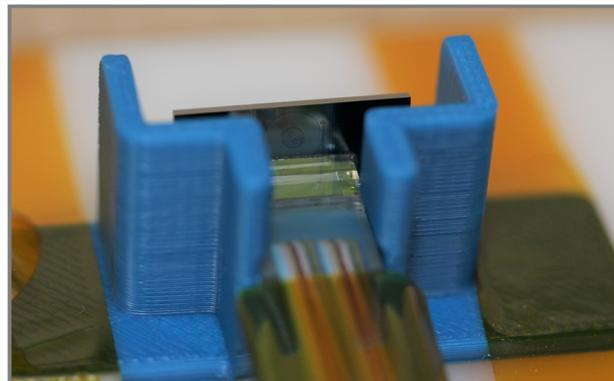
**Figure 2:** The 6x6 mm PIC is attached to a 1x48 V-groove fiber array using UV adhesive. The fiber array is bedded in a 3D printed holder, with the PIC suspended by the adhesive. Note the multimode spiral waveguide.
