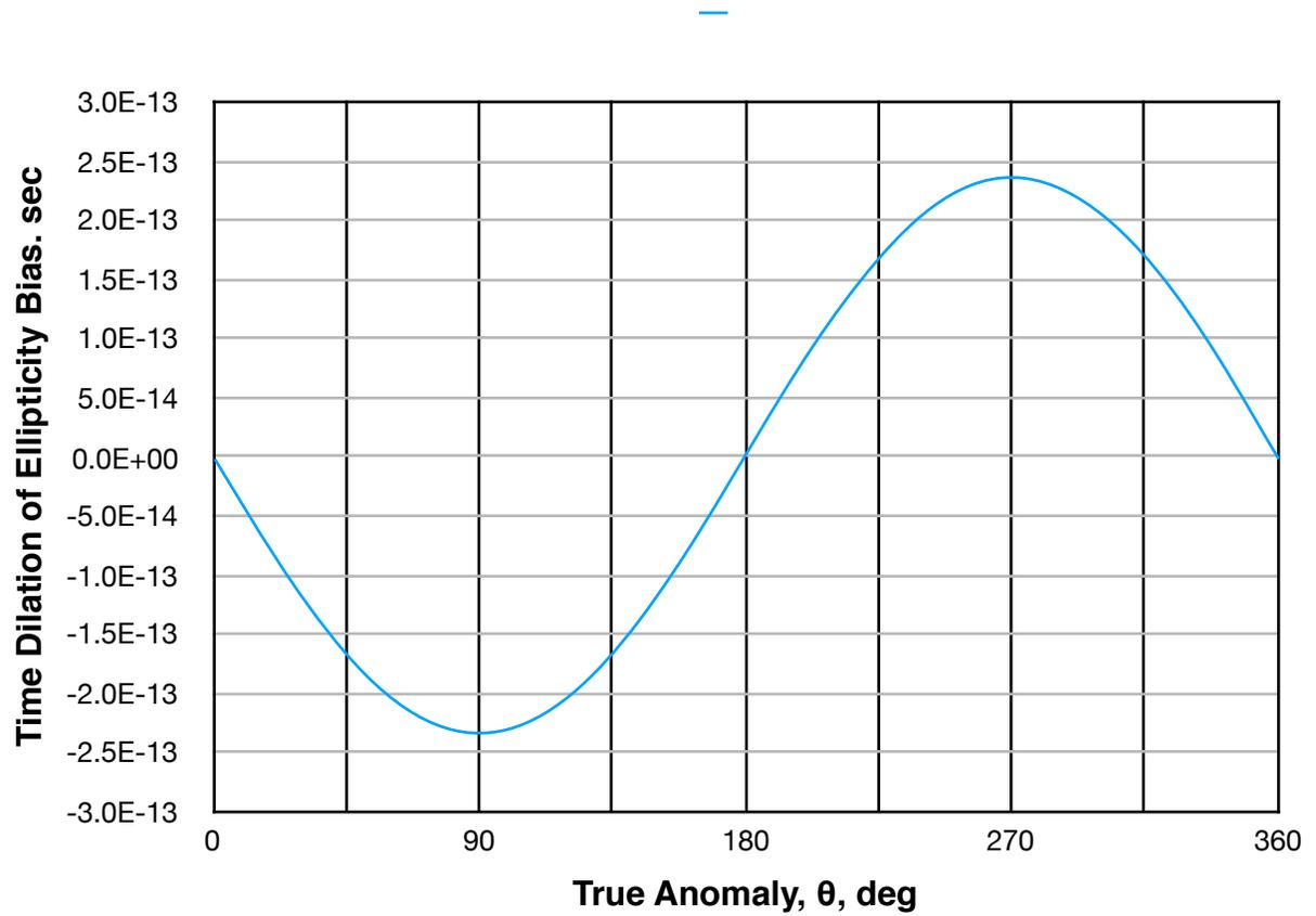
**Figure 1. Time Dilation Difference, Vector Minus Algebraic Calculation with Ellipticity of 0.001**
