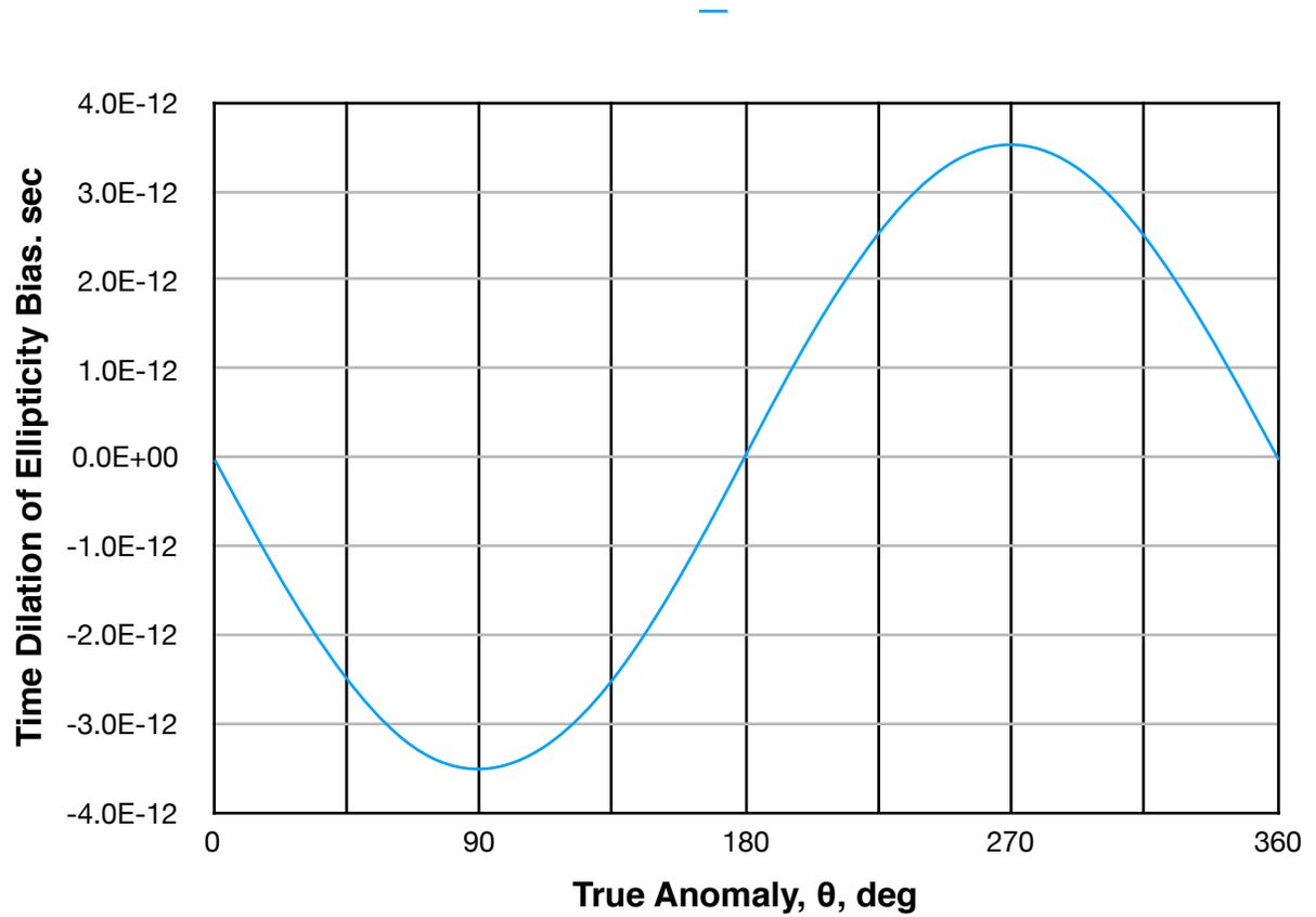
**Figure 3. Time Dilation Difference, Vector Minus Algebraic Calculation with Ellipticity of 0.015**
