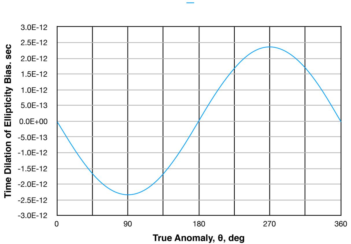
**Figure 2. Time Dilation Difference, Vector Minus Algebraic Calculation with Ellipticity of 0.01**
