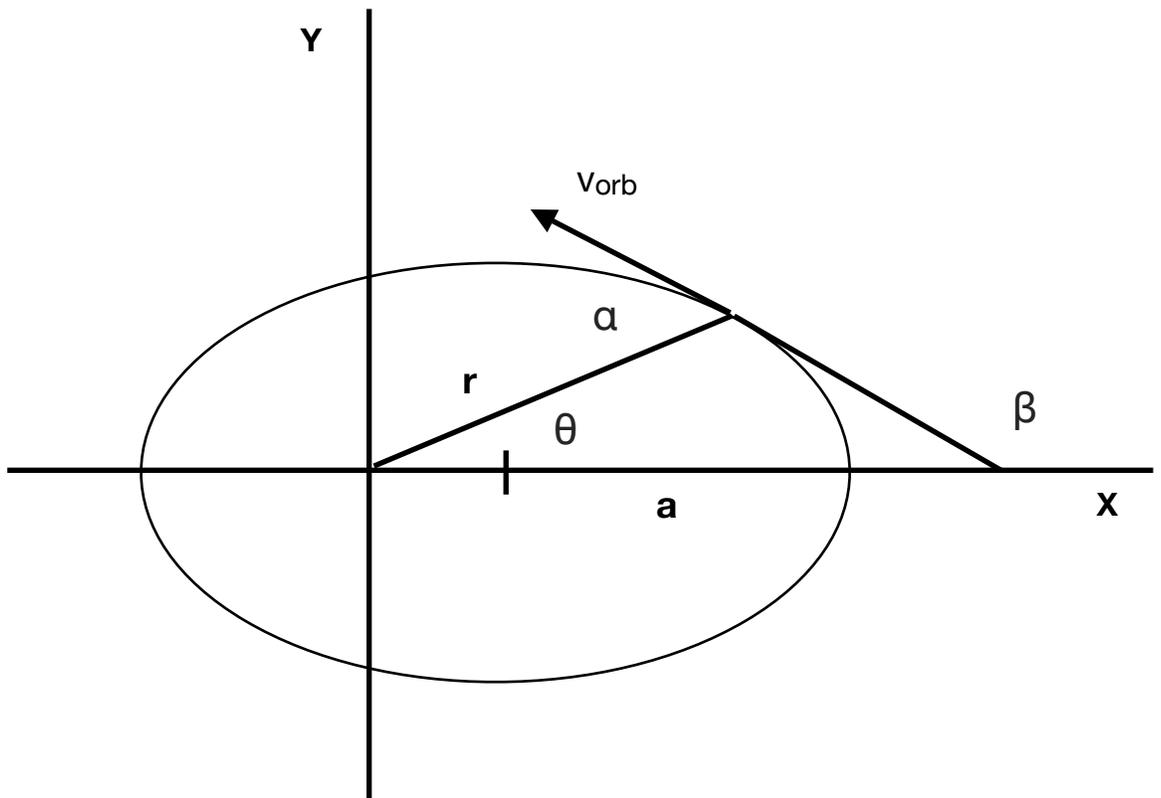
**Figure B.1 Elliptical Orbit Parameters
