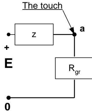
**Fig. 1:** Our equivalent scheme. "Z" is our " $R_{int}$ ". The generator is thus {E,Z}. E here is 220V. Point a denotes the metal body of the generator, which can be touched by the student, and where, in the case of the fault, a dangerous voltage arises.
