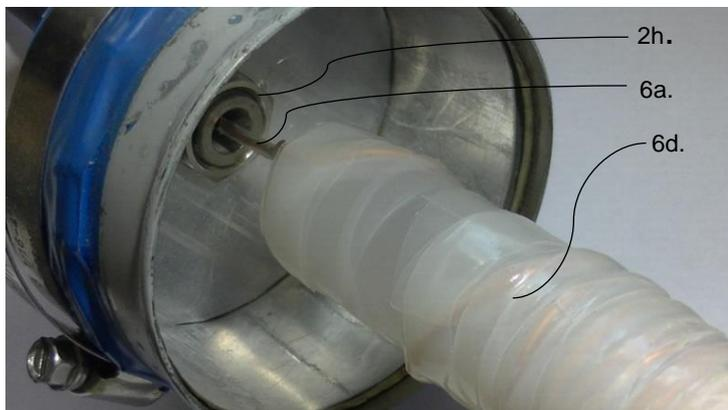
**Image 2:** N-type female bulkhead (2h.), aerial wire leading to solenoid (6a.), proxy-aerial (6d).
