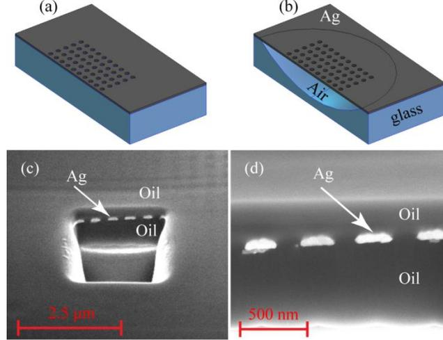
Fig. 2: Cross-sectional schematics of the array (a) before and (b) after etching with HF. (c) cross-sectional SEM image of the freestanding array in a homogenous dielectric environment (immersion oil). (d) Close-up of (c).
