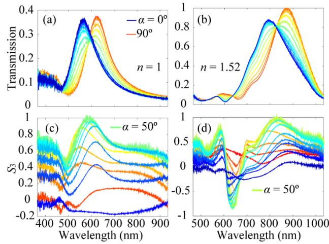
Fig. 3: Experimentally obtained results for incident polarization  $0^\circ \leq \alpha \leq 90^\circ$ . Normalized transmission vs. the wavelength for (a)  $n = 1$  and (b)  $n = 1.52$ .  $S_3$  vs. the wavelength for (c)  $n = 1$  and (d)  $n = 1.52$ .
