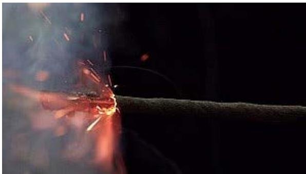
Detonating cord burning in one direction.
