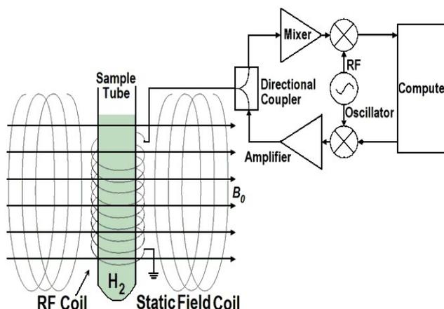
**Fig.17.** Simplified experimental NMR-like resonance apparatus for putative LSXD C-QED ionization of TBS in hydrogen. The Fig. only shows possible details for rf-modulating TBS QED resonance, not the spectrographic recording and analysis components.
