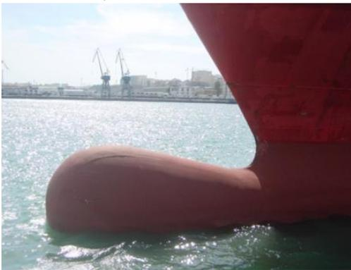
Nowadays, big ships and also small ones, have the lower part that is submerged, a bulb in the front. The function of this bulb is to create a series of waves or turbulence, which when joined with the waves generated by the boat itself, are annulled or at least almost eliminated. In this way, they greatly reduce the drag of the boat.
