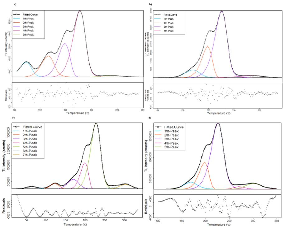
Fig. 2. Glow curve deconvolution of MTS600 treated with no preheat at 1 Gy (FOM: 0.72%) and 50 Gy (FOM: 0.55%) a), c) and MTS600 treated with preheat at 1 Gy (FOM: 0.83%) and 50 Gy (FOM: 0.30%) b), d) representatively.
