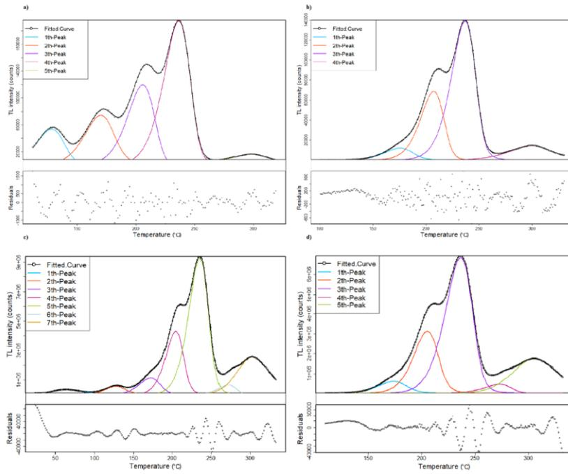
Fig. 1. Glow curve deconvolution of MTS100 treated with no preheat at 1 Gy (FOM: 0.52%) and 50 Gy (FOM: 0.52%) a), c) and MTS100 treated with preheat at 1 Gy (FOM: 0.63%) and 50 Gy (FOM: 0.63%) b), d) representatively.
