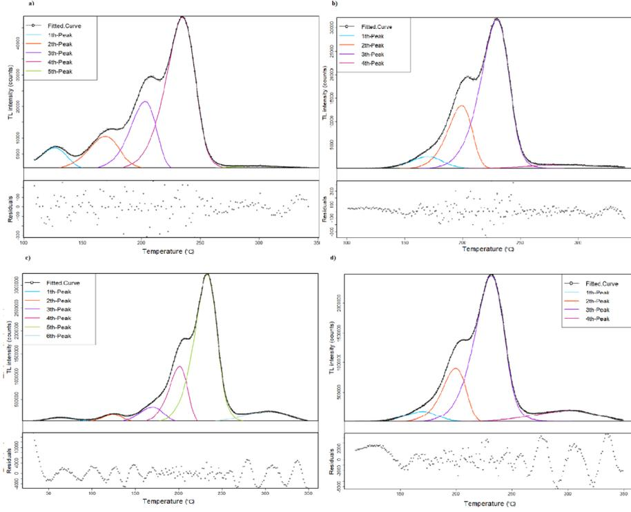
Fig. 3. Glow curve deconvolution of MTS700 treated with no preheat at 1 Gy (FOM: 0.65%) and 50 Gy (FOM: 0.35%) a), c) and MTS700 treated with preheat at 1 Gy (FOM: 0.92%) and 50 Gy (FOM: 0.30%) b), d) representively.
