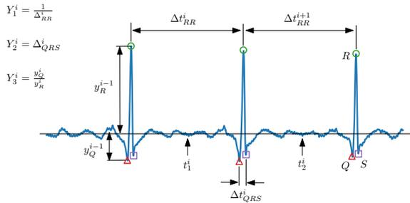
**FIGURE 3.** Statistical ECG features of interest extracted from the sensor ECG signal
