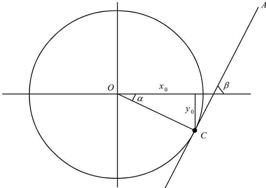
**Drawing 2.-** The circumference is the Moon, and the line  $A-C$  is the tangent to the lunar surface at point  $C$ .
