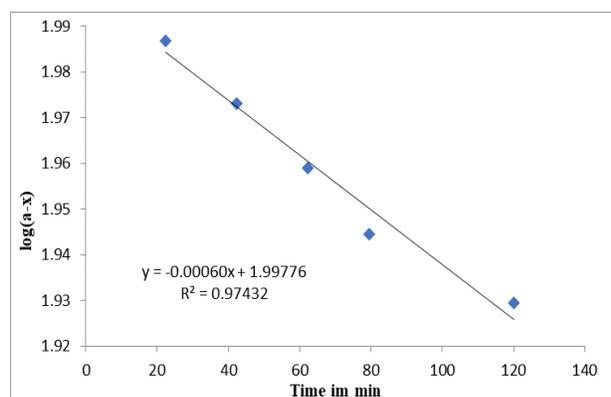
Fig. 1: Plot of log(a-x) versus time at [KIO<sub>4</sub>] = 0.002 M, [PEG-400] = 0.025M, [OH<sup>-</sup>] = 0.1 M and Temperature = 35 °C
