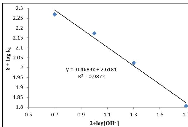
Fig. 2. Effect of alkali concentration on oxidation of PEG-400 by periodate
