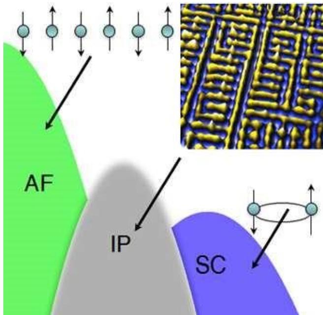
An "antiferromagnetic" state, where the magnetic moments of electrons are opposed, can lead to a variety of unexpected arrangements of electrons in a high-temperature superconductor, then finally to the formation of "Cooper pairs" that conduct without resistance, according to a new theory. [22]
