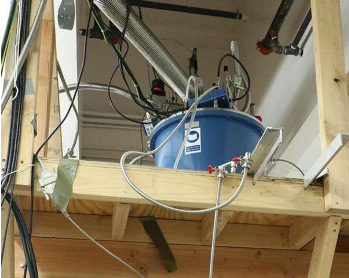
Optical dilution refrigerator for low-temperature experiments at UC San Diego. Credit: Michelle Fredricks
