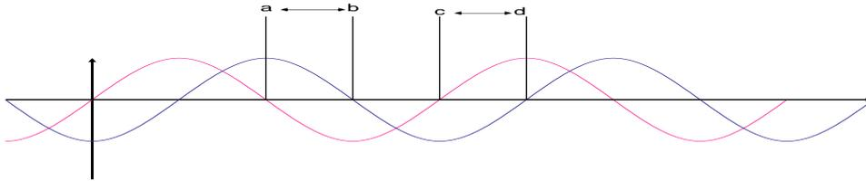
Fig 4 | Plot of the Electric or Magnetic fields of two unified waves that had a phase shift relative to one another
