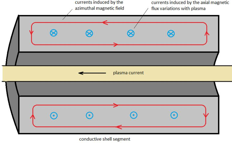
Figure 2.4: Section view through one segment of the conductive shell
