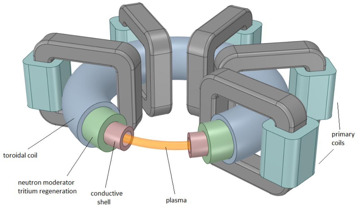
Figure 2.1: Electrodynamic stabilization the structure of principle
