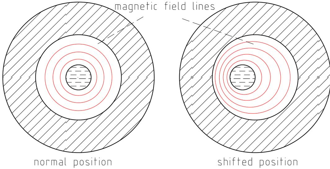
Figure 2.3: Plasma levitation inside the metallic shell
