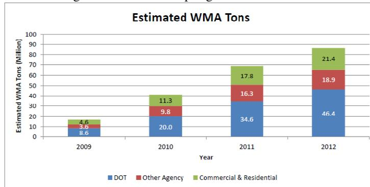
Figure 5 Growth of Warm Mixed Asphalt Usage per year (2009-2012) in USA [9]
