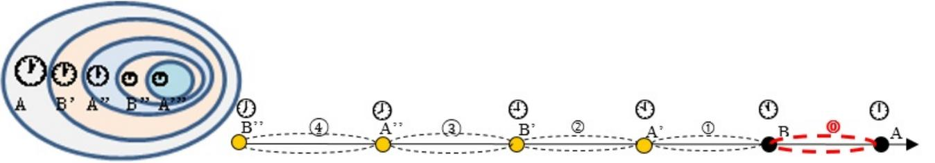
**Figure 2.** Recursive mirroring: two mirrors facing each other are reflected recursively. If there is a clock on each of them, from the reflected image present in every instant it is possible to reconstruct distances historically and therefore the velocities and accelerations over time, as far as the reflection allows.
