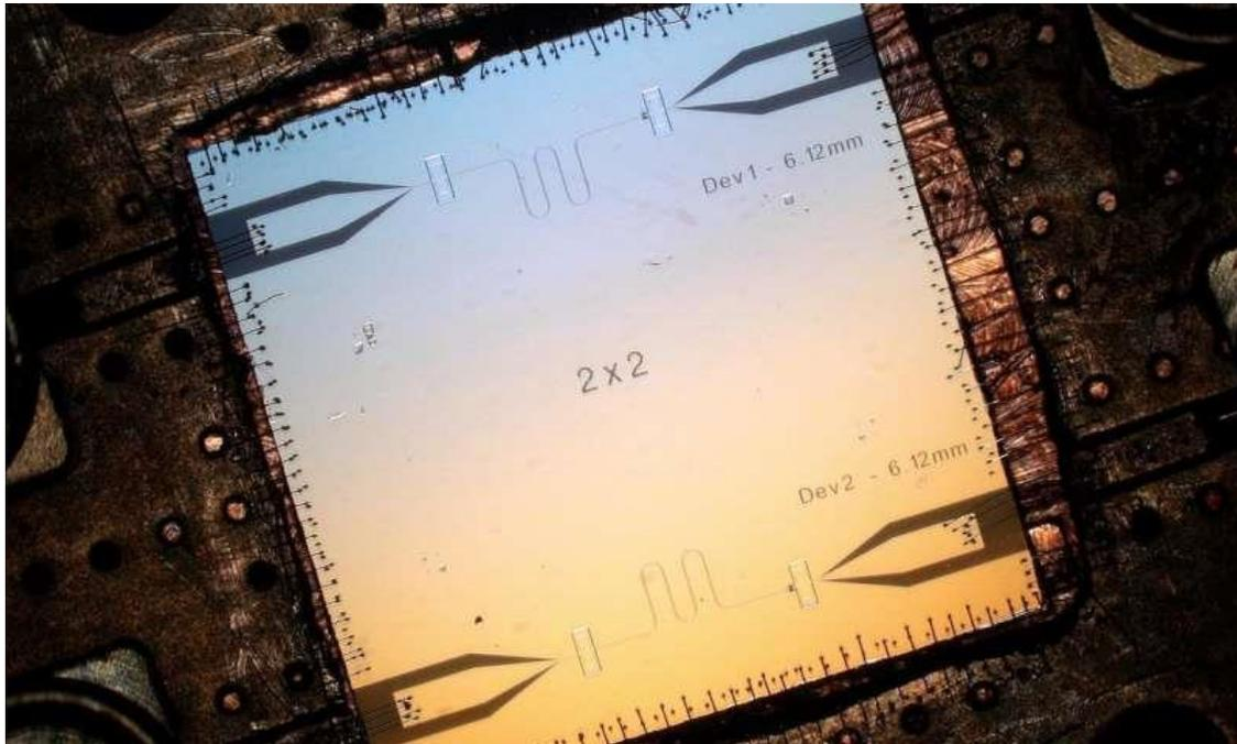
Close-up of the new a superconducting microwave circuit with a graphene Josephson junction.
