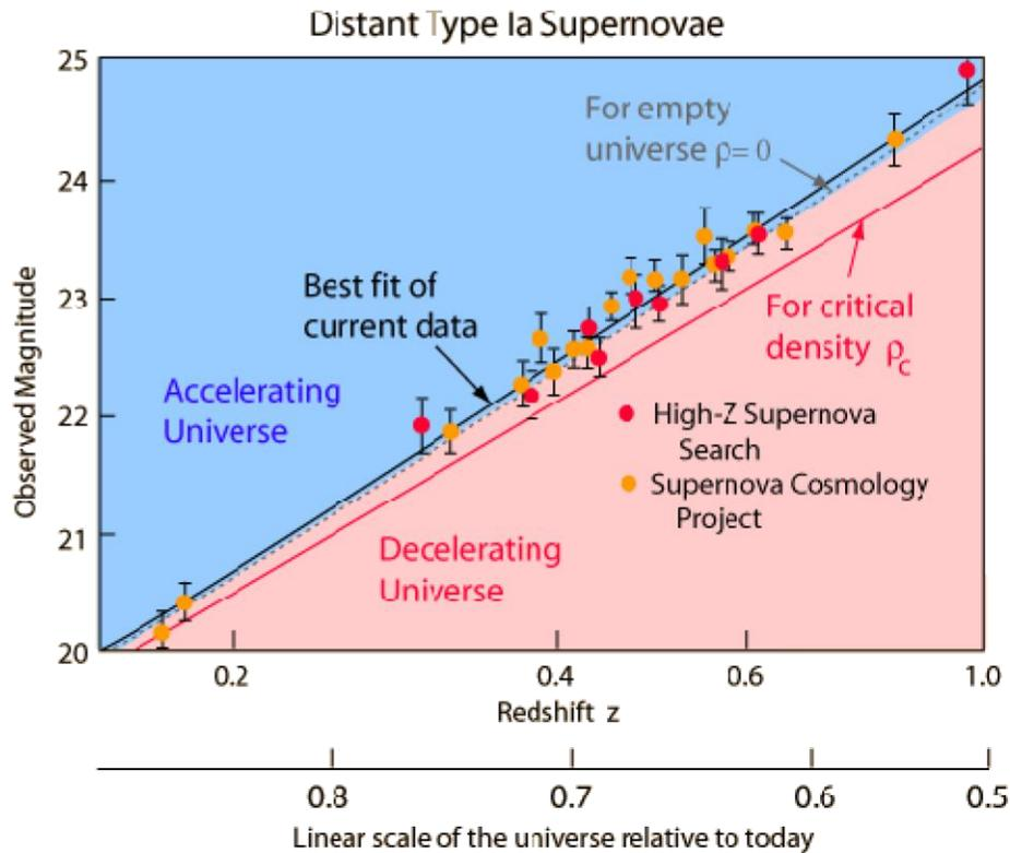
The data summarized in the illustration above involve the measurement of the redshifts of the distant supernovae. The observed magnitudes are plotted against the redshift parameter  $z$ . Note that there are a number of Type Ia supernovae around  $z=0.6$ , which with a Hubble constant of 71 km/s/mbpc is a distance of about 5 billion light years.
