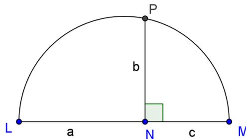
Fig. 2. b gives the mean proportional of the quantities a and c.
