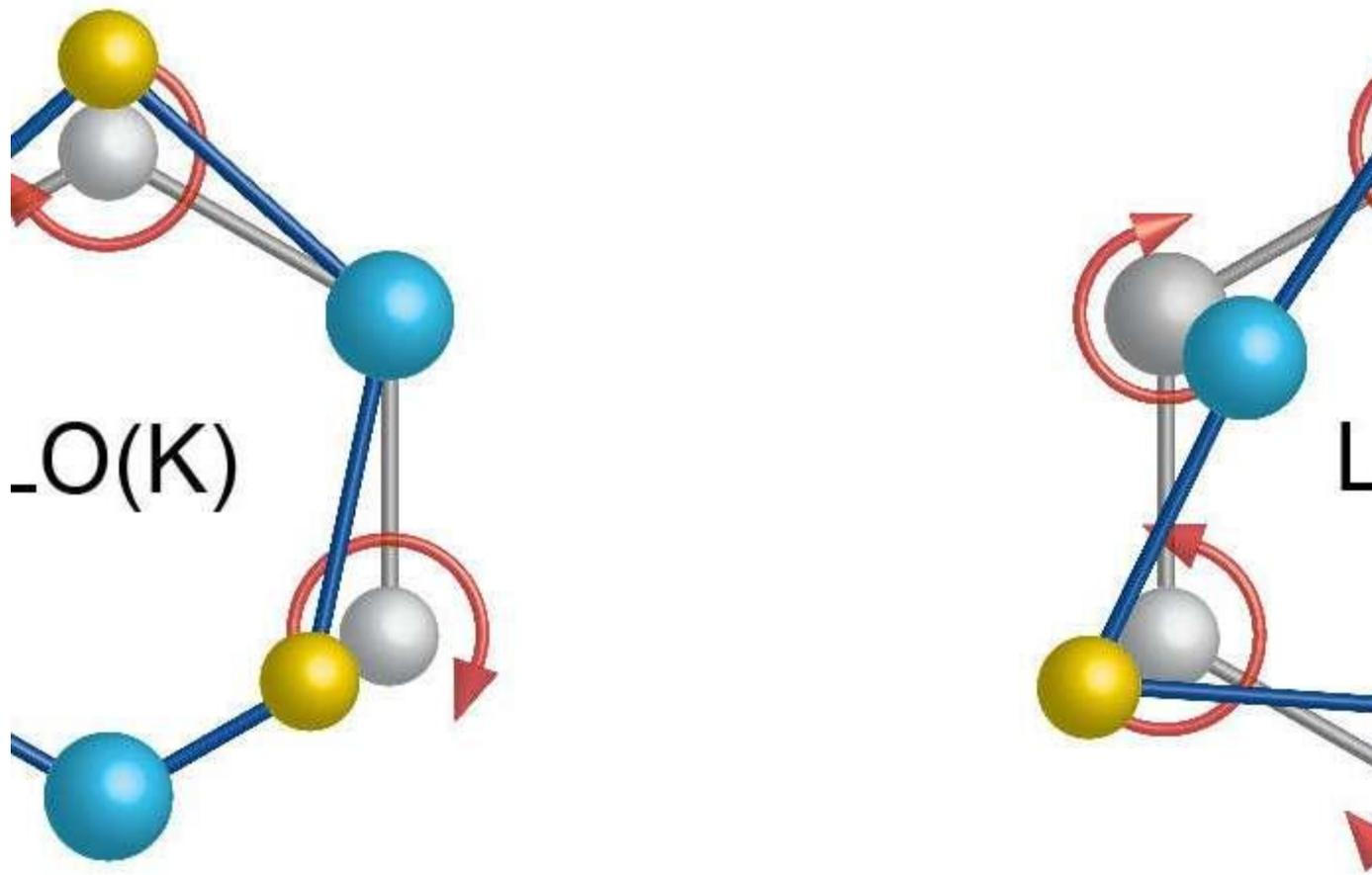
This diagram maps out atomic motion in separate phonon modes. At left ("LO" represents a longitudinal optical mode), selenium atoms exhibit a clockwise rotation while tungsten atoms stand still. At right ("LA" represents a longitudinal ...[more](#)
