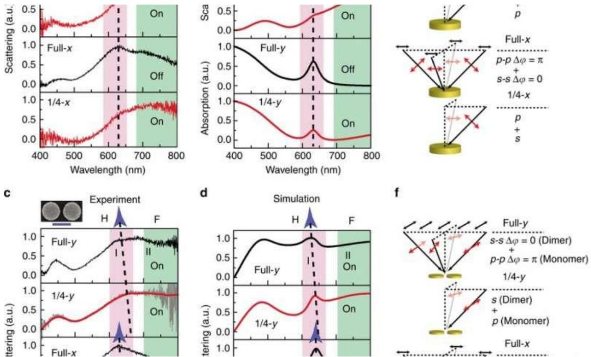
Demonstration of plasmonic switching by dark field (DF) scattering measurement of gold nanodisk monomer and dimer. a Normalized DF scattering spectra of gold nanodisk monomer with a diameter of 200 nm (SEM image) under full and quarter ...[more](#)
