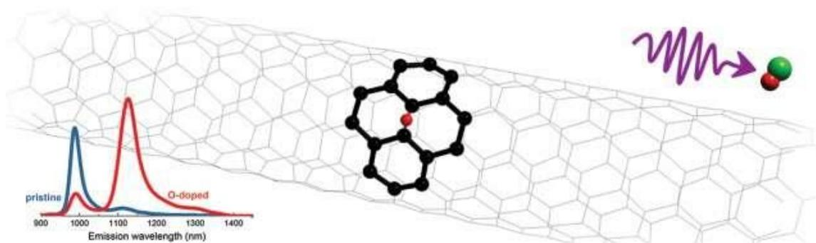
Submerging a carbon nanotube in bleach produces an oxygen atom (red) that reacts with the carbon atoms (black) of the nanotube, forming a fluorescent quantum defect when irradiated with ultraviolet light. Credit: Belcher Lab
