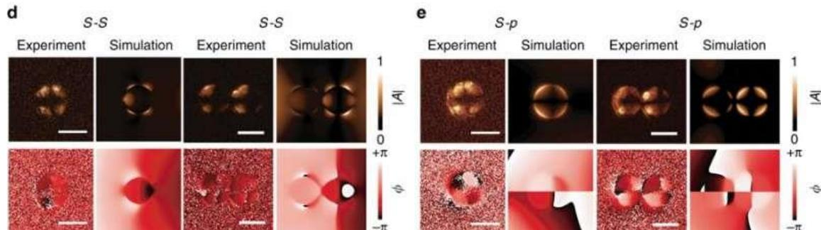
Demonstration of electrical-field distribution rule for the 200 nm gold nanodisk monomer and dimer by s-SNOM. a Schematic of the s-SNOM measurement for s-s and s-p excitation-collection configurations. The wavelength of the excitation laser [...more](#)
