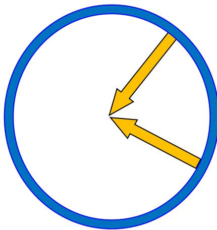
Object moving in circle with constant speed has acceleration toward the middle of the circle
