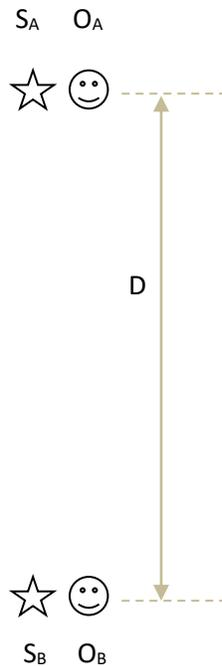
As before, if A and B are at absolute rest, the round trip time of light will be  $2D/c$ , hence the frequency of the pulses will be  $f = 1/(2D/c) = c/2D$ .
