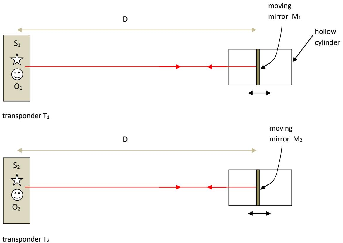
The motions of the mirrors in the two setups are  $180^{\circ}$  out of phase. When one mirror is moving to the left the other is moving to the right, and vice versa.
