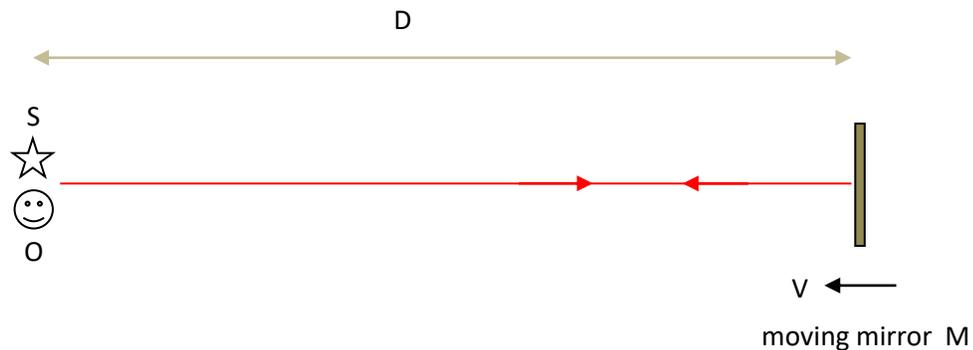
Initially, a short light pulse is emitted by the light source S. Light reflected from the moving mirror is detected by detector O. Detector O, upon detecting the light pulse, immediately triggers source S, upon which S emits another light pulse and the cycle continues. An electronic counter counts the number of pulses detected (or emitted ).
