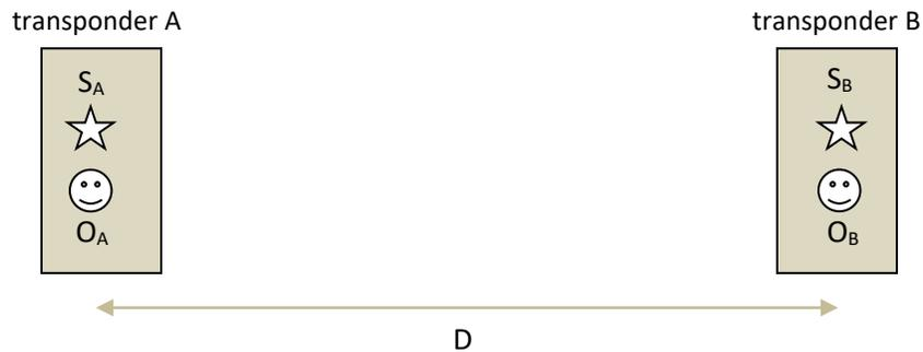
Initially  $S_A$  emits a short light pulse, which will be detected by  $O_B$ , which will trigger  $S_B$  to immediately emit a short light pulse, which will be detected by  $O_A$ , which will trigger  $S_A$  to
