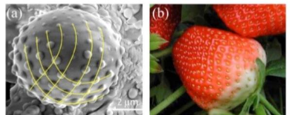
FIG. 4. Parastichous spirals on frustrating surfaces. (a) Stressed pattern on a slanted Ag core/SiO<sub>2</sub> shell microstructure, and (b) the "X pattern" of achenes in a strawberry.
