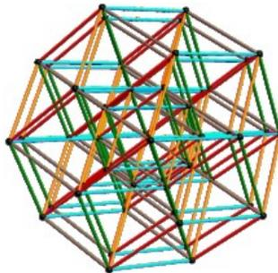
A **6-cube** projected into the rhombic triacontahedron using the golden ratio in the basis vectors. **This is used to understand the aperiodic icosahedral structure of quasicrystals**
