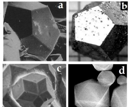
**Fig 2 :** a.) Dodecahedral Quasicrystal **Al<sub>65</sub>Cu<sub>20</sub>Fe<sub>15</sub>**
