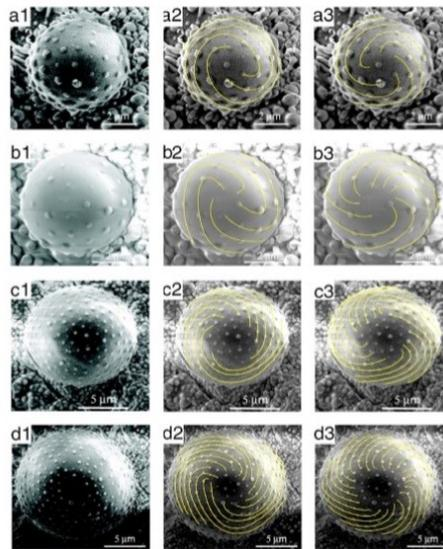
**FIG. 1.** Fibonacci spiral patterns in the sinister form grown on Ag-core/SiO<sub>2</sub> shell microstructures: (a) 3x5, (b) 5x8, (c) 8x13 and (d) 13x21.
