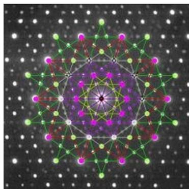
A **5-cube** as an orthographic projection into 2D using Petrie polygon basis vectors overlaid on the diffractogram from an icosahedral Ho-Mg-Zn quasicrystal
