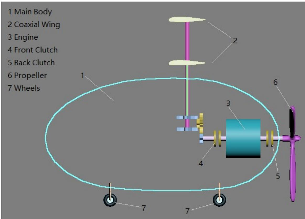
Figure 2: Components of Lin's Helicopter
