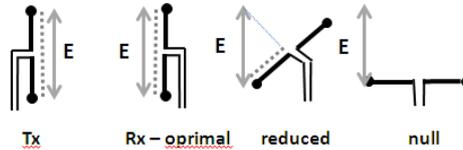
Figure 1. Comparison of conventional dipole transceiver antennas positioning.
