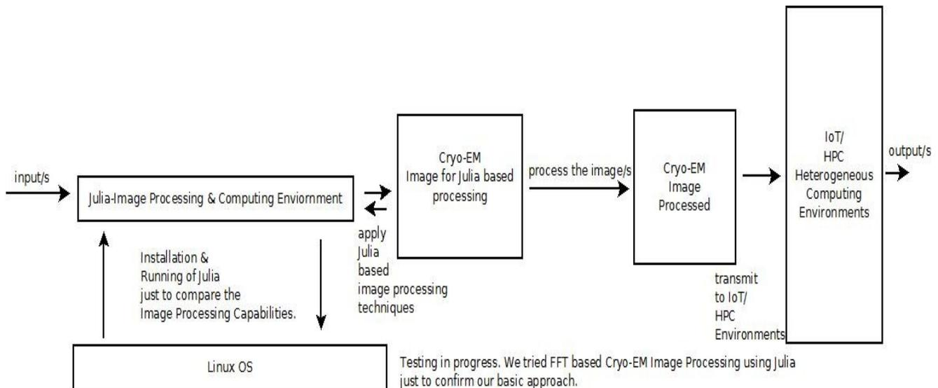
Approximate Algorithm for Cryo-EM Image Processing Using Julia alone With MXNet/Flux ML Libraries.
