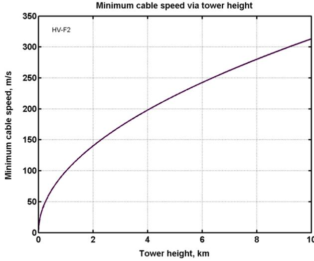
Fig. 5.8. Minimum cable speed via tower height.
