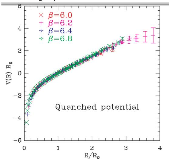
The static  $q\bar{q}$  potential in the quenched approximation obtained by the Wuppertal collaboration. The data at  $\beta = 6.0, 6.2, 6.4$  and  $6.8$  has been scaled by  $R_0$ , and normalized such that  $V(R_0) = 0$ . The collapse of the different sets of data on to a single curve after the rescaling by  $R_0$  is evidence for scaling. The linear rise at large  $r$  implies confinement. [9]
