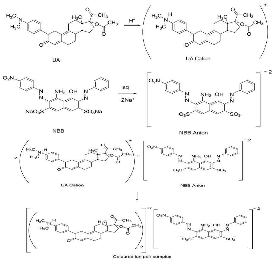
Fig. 5. Reaction of Ulipristal acetate with naphthol blue black
