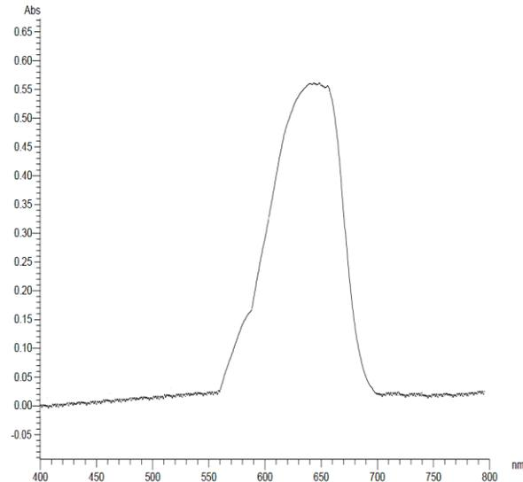
Fig. 2. Visible spectrum of UPA-NBB ion-association complex
