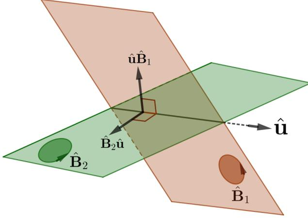
Figure 2: The vector  $\hat{\mathbf{u}}\hat{\mathbf{B}}_1$  is parallel to the bivector  $\hat{\mathbf{B}}_1$ , and the vector  $\hat{\mathbf{B}}_2\hat{\mathbf{u}}$  is parallel to the bivector  $\hat{\mathbf{B}}_2$ . Both vectors are  $90^\circ$  rotations of the vector  $\hat{\mathbf{u}}$ , but are not necessarily perpendicular to each other. Instead, the angle between them is equal to the angle between the two planes.
